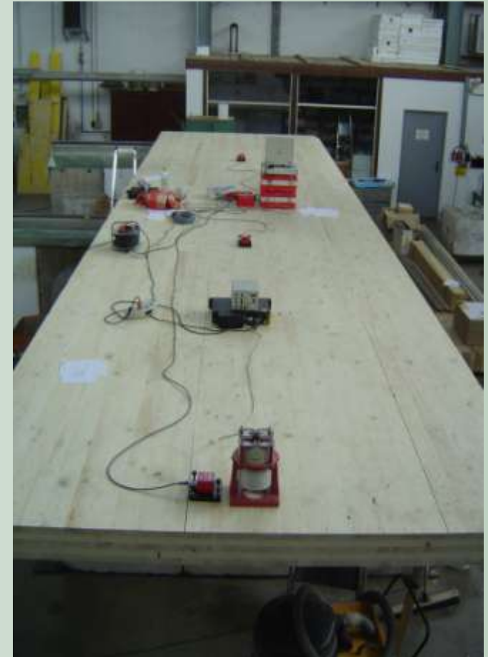
continuous beam with cantilever and measurement equipment (cont;clt|-)
