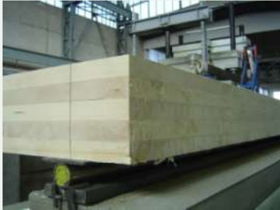
5-layered CLT element (clt|-)
