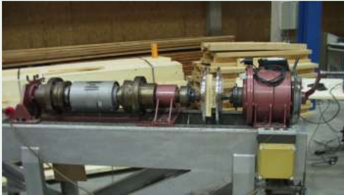
torsional test configuration
