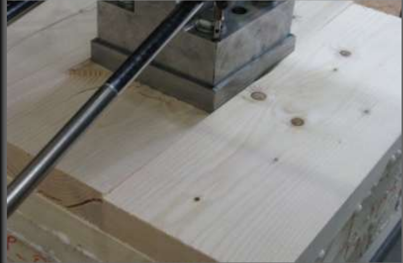
compression perp.to grain | TU Graz
