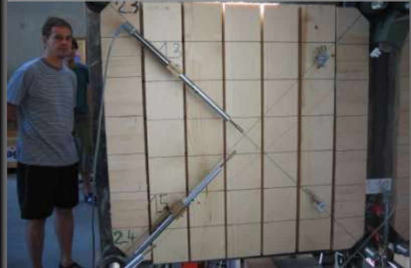
slab shear tests | TU Graz
